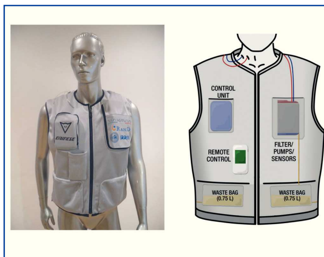
Figure 2. WAKMAN project: a complete system for the ambulatory treatment of congestive heart failure.
